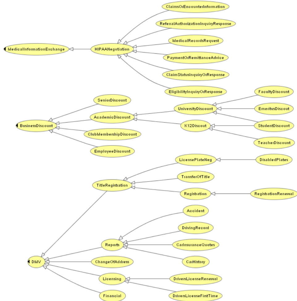
Figure 7.3: The class hierarchy graphically representing is a properties between classes for three trust negotiation ontologies. Other class interrelationships, such as the property hasTypicalAttribute , are not shown. The complete ontology description is included in Appendix A.
